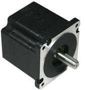
The 34Y112S-LW8-MS High Torque Stepper Motor offers a great value without sacrificing quality. This motor was designed to offer the highest possible torque while minimizing vibration and audible noise. It is wired in series with a Molex 4 pin Mini-Fit Jr. receptacle.
